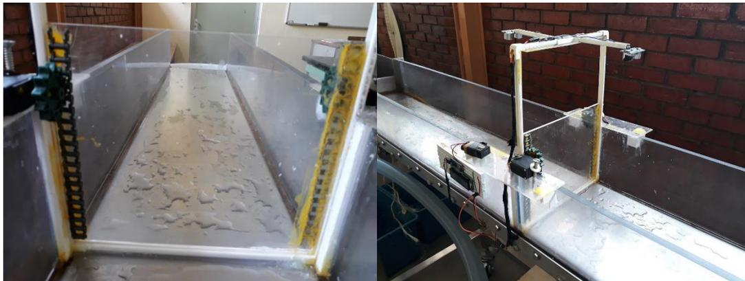
**Figure 2.** Acrylic electro-gate in the channel
